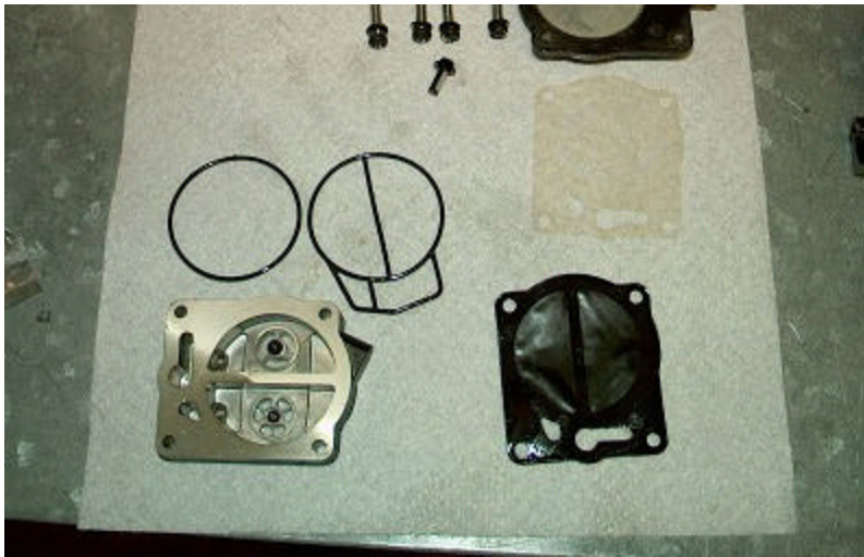
Components of pump side, strainer, o-rings, diaphragms, pump body and cover
