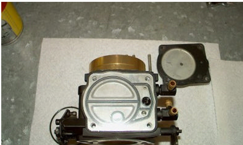
Install corresponding o-ring in correct position and strainer
